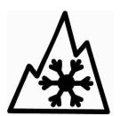
Sidewall symbol for Severe Snow Use Tires typically placed adjacent to the M+S type designation. Minimum 15 mm/0.6" base and 15 mm/0.6" height.
