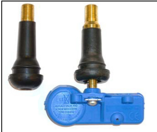
FIGURE 4A: Comparing Standard Snap-In Valve to a TPMS Snap-In Valve with Sensor
