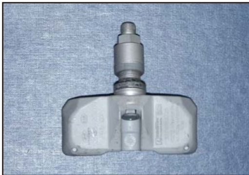
FIGURE 4C: Clamp-in TPMS Valve
