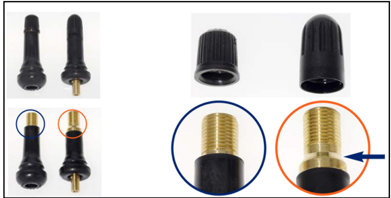
FIGURE 4B: Comparison: Valve Cap and Valve Tip Close-Up Above are the same photos comparing standard valves and TPMS valves with and without their valve caps. Note the larger tapered shoulder on the sensor valve of the TPMS.
