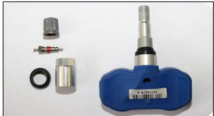
FIGURE 4D: TPMS Replacement Kit with Valve Assembly
