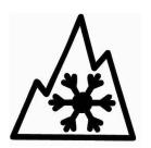
Sidewall symbol for Severe Snow Use Tires to be placed adjacent to the M+S type designation. Minimum 15 mm/0.6" base and 15 mm/0.6" height.
