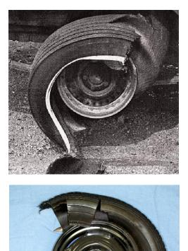
The centrifugal forces created by a rapidly spinning tire can cause an explosion by literally tearing the tire apart. These forces act on the complete tire structure and can be of such magnitude as to break the beads, in addition to, rupturing the tire. Some vehicles are able to bring a tire to its centrifugal force failing point in just 3 to 5 seconds.
