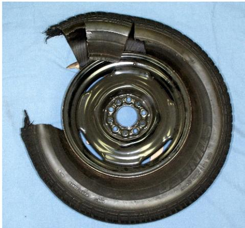
The centrifugal forces created by a rapidly spinning tire can cause an explosion by literally tearing the tire apart. These forces act on the complete tire structure and can be of such magnitude as to break the beads, in addition to, rupturing the tire. Some vehicles are able to bring a tire to its centrifugal force failing point in just 3 to 5 seconds.
