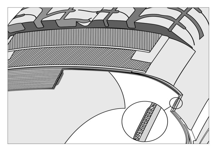
Sidewall indentations are a cosmetic characteristic and will not affect the performance of the tire. If bulges, rather than indentations, appear on the sidewall or if there is any question concerning the sidewall appearance, the tire should be examined by a tire service professional.
