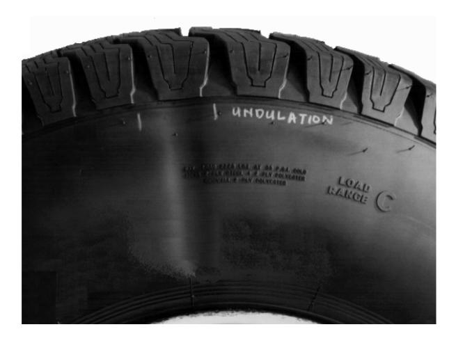
The condition, sometimes referred to as sidewall undulations, is a common characteristic of radial tire construction. These indentations are more noticeable in tire sizes with higher aspect ratios and/or higher inflation pressures.
