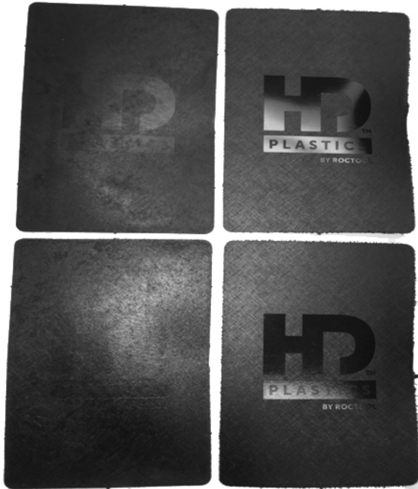
(top) 8099 MRP-filled resin (bottom) 4080 MRP-filled resin (left) conventional injection molding (right) induction-heated molding
