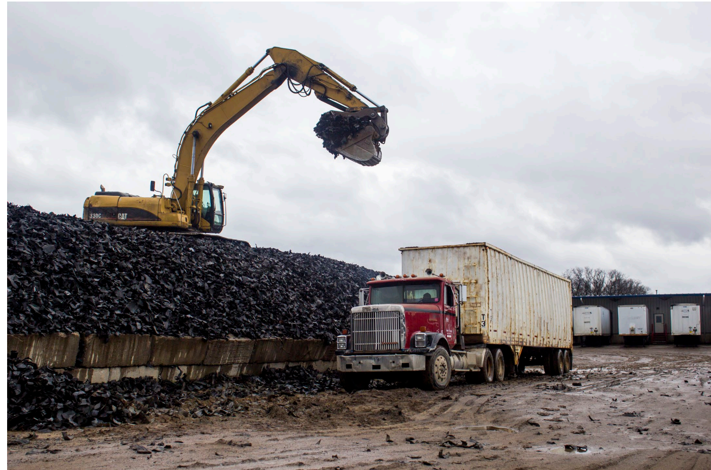
Manufactured TDA Storage bins and Loading Equipment.
